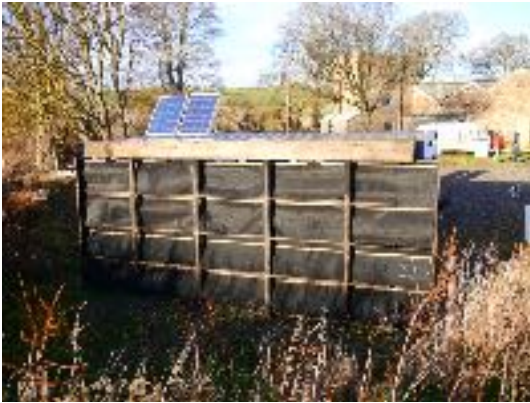
Fig.2 Front of kiln with heat absorbing mesh
